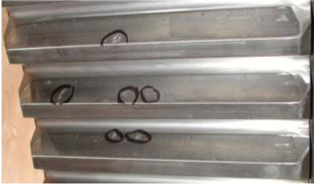
Fig. 2. Photo of tooth pitting
