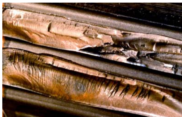
Fig. 1. Photo of tooth cracking
